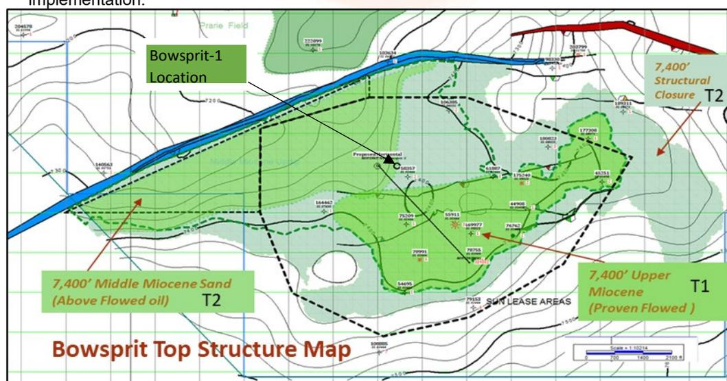
Figure 1- Bowsprit Field segments and approximate well path
