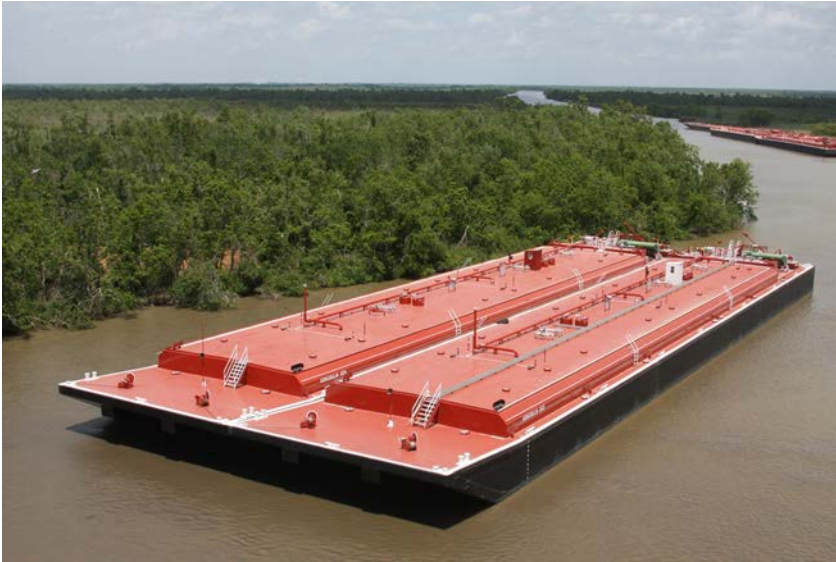
Shallow-draft export / storage barge
