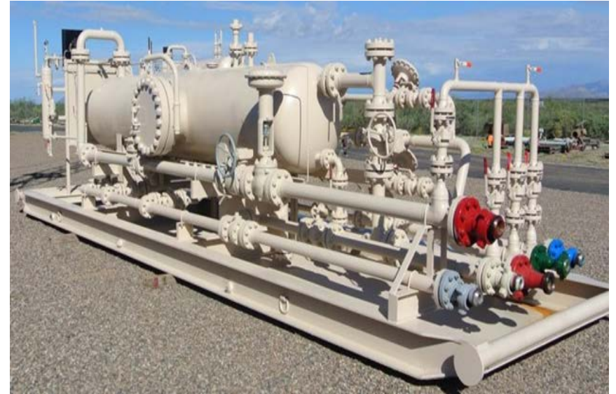
Modular Separator to place on moored barge or old jack up for low cost development
